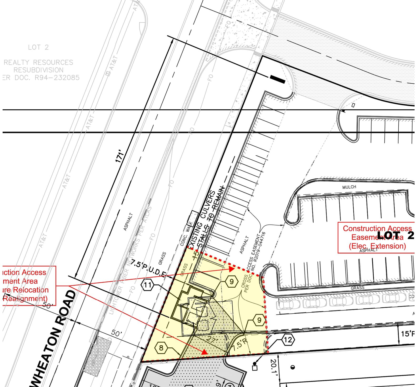
Construction Access Easement Area (Fire Relocation Realignment)
