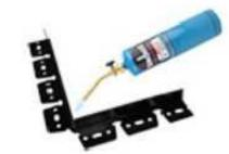
Since our paver restraints are made of true PVC, they can be heated with a propane torch or heat gun and then bent to form 90 degree corners and other angles. Be sure to practice your technique on scrap pieces before applying it in the field.
