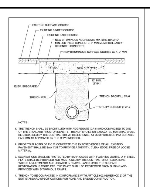
City of Naperville UTILITY TRENCH PAVING SECTION PAVEMENT 13
