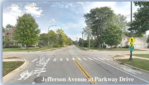
There is a one-sided, west-facing Pedestrian Crossing assembly (W11-2, W16-7P) on the south side of Jefferson Avenue directly at the crosswalk and a one-sided, east-facing Pedestrian Advance Crossing assembly with AHEAD plaque on the north side of Jefferson Avenue to the east of the intersection. There is also an east-facing School sign (S1-1) further to the east on Jefferson Avenue. The School Walk Route plan for WJHS directs students to cross both approaches of Parkway Drive.
