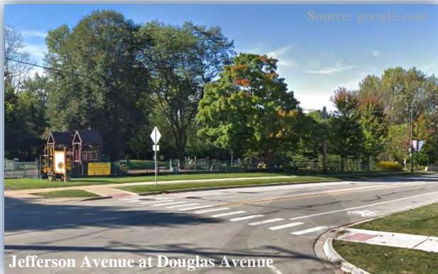
a one-sided, west-facing Pedestrian Crossing assembly (W11-2, W16-7P) on the south side of Jefferson Avenue directly at the crosswalk and a one-sided, east-facing Pedestrian Crossing assembly on the north side of Jefferson Avenue to the east of the intersection. There are also Pedestrian Advance Crossing assemblies with AHEAD plaques posted in both directions on Jefferson Avenue in advance of the crosswalk. The Douglas Avenue crossing is part of the School Walk Route plan for WJHS.
