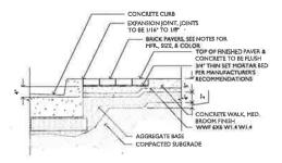
BRICK AND CONCRETE PAVING
