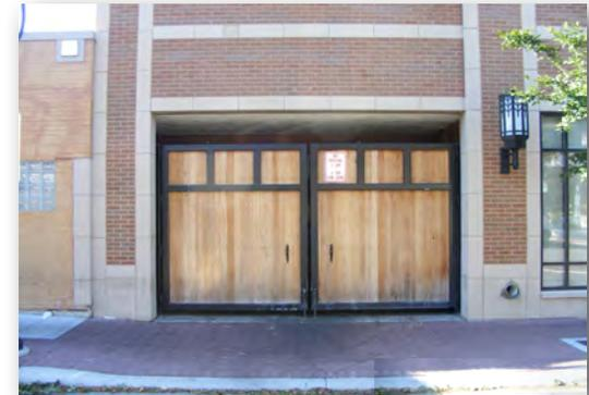
**Image 23:** Refuse storage areas may be inset into a building facade and screened with opaque fencing.
