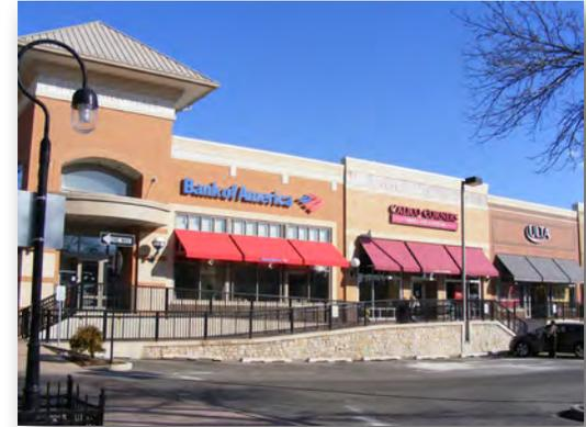
**Image 4:** Variations in the exterior wall plane subdivide the facade on this single building into multiple vertical storefront segments
