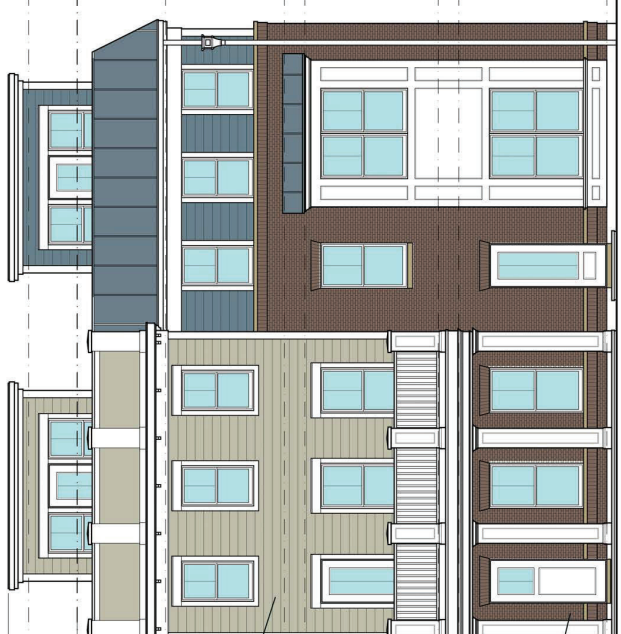
Unit 13 Duplex II — Front Elevation (West) SCALE: 1/4" = 1'-0"
