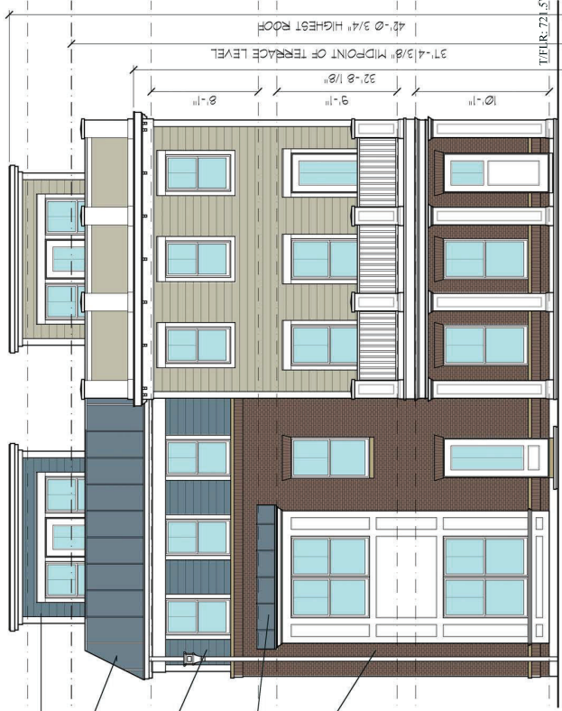
Unit 10 1 Duplex I - Front Elevation (East-Loomis) SCALE: 1/4" = 1'-0"
