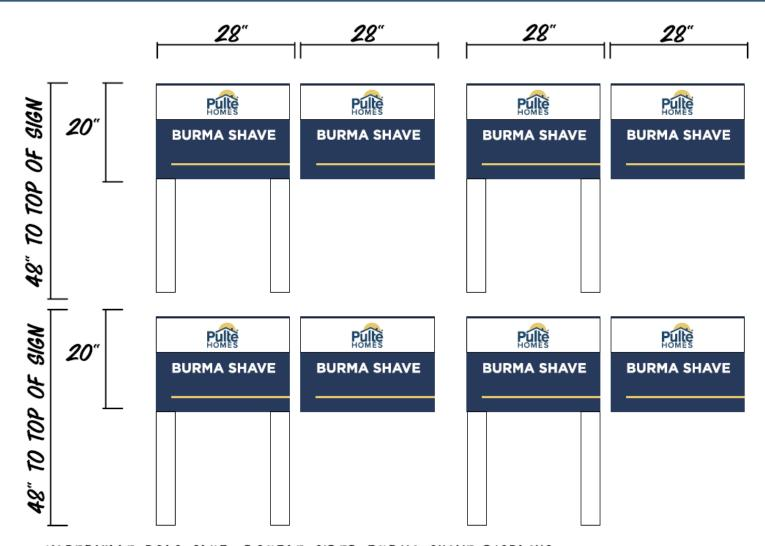
NAPERVILLE POLO CLUB: DOUBLE-SIDED BURMA SHAVE DISPLAYS-3/8" MDO w/ WHITE VINYL COPY & DIGITALLY PRINTED DETAIL MOUNTED TO (2) 4" X 4" WOOD POSTS- PAINTED WHITE EXACT COPY & INSTALLATION LOCATIONS TO BE DETERMINED
