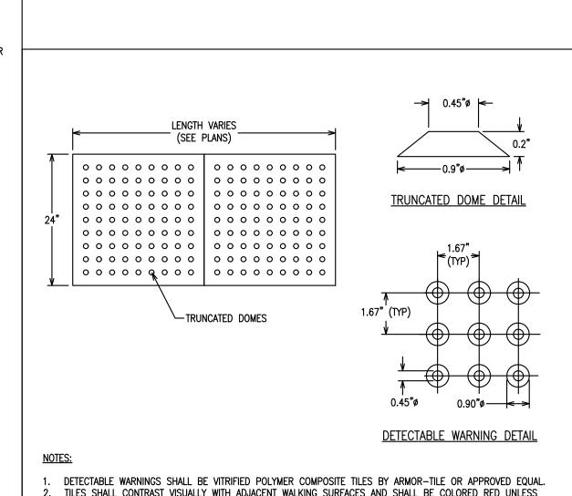
TILES SHALL CONTRAST VISUALLY WITH ADJACENT WALKING SURFACES AND SHALL BE COLORED RED UNLESS OTHERWISE DIRECTED BY LOCAL BUILDING CODES. 3. TILES SHALL BE INSTALLED IN ACCORDANCE WITH MANUFACTURER'S SPECIFICATIONS AND RECOMMENDATIONS.
