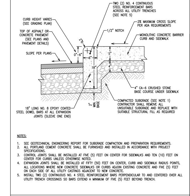
MONOLITHIC CONCRETE CURB AND SIDEWALK DETAIL
