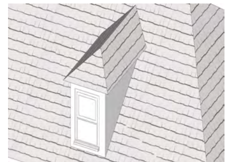
Illustration D.22 - Hipped dormer example
