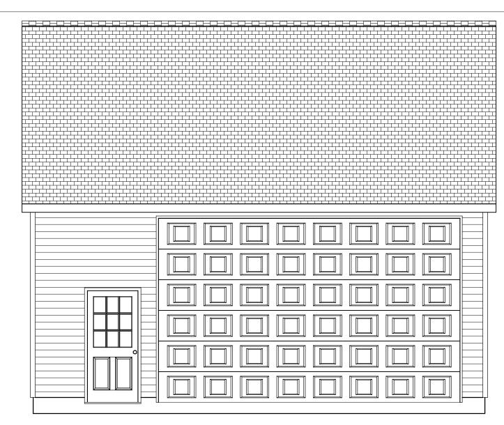
The garage is 22'4" from the top of the foundation to the roof peak.
