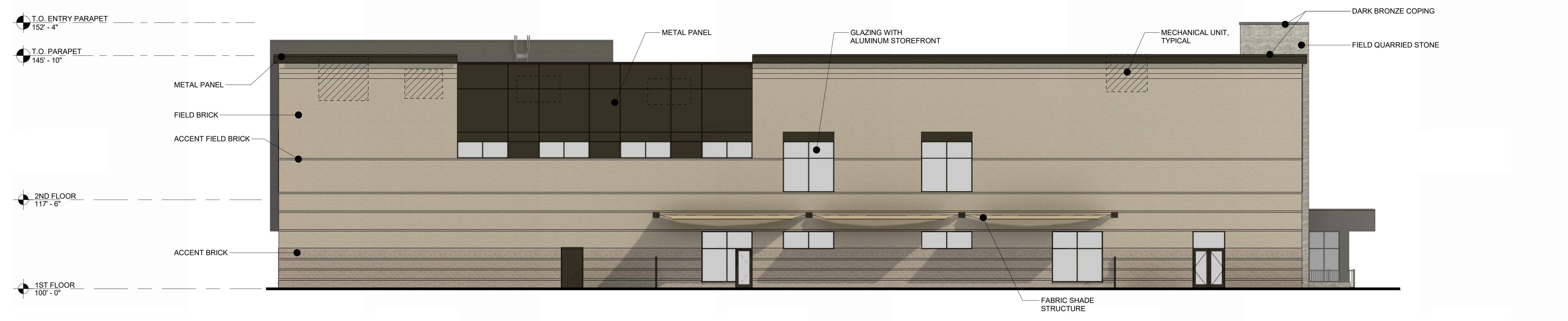
2 EXTERIOR ELEVATION - EAST 3/32" = 1'-0"
