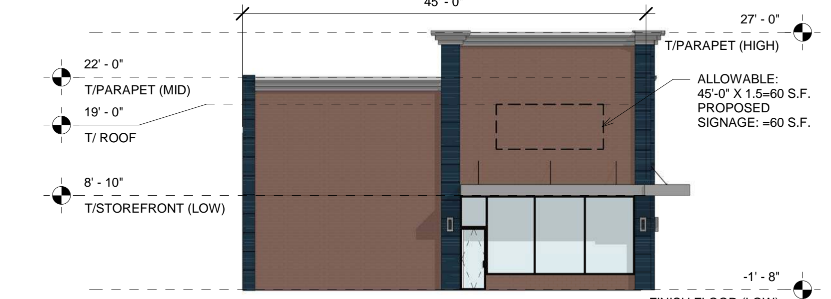
5 PROPOSED FACADE RENOVATION - EAST ELEVATION 3/32" = 1'-0"
