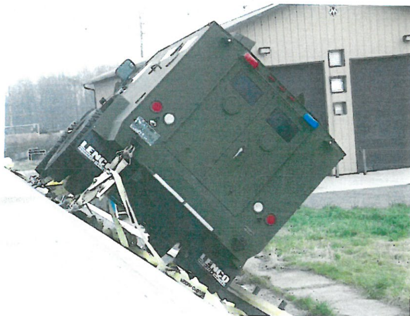
Figure 6. BearCat on the Tilt Table at rollover threshold.
