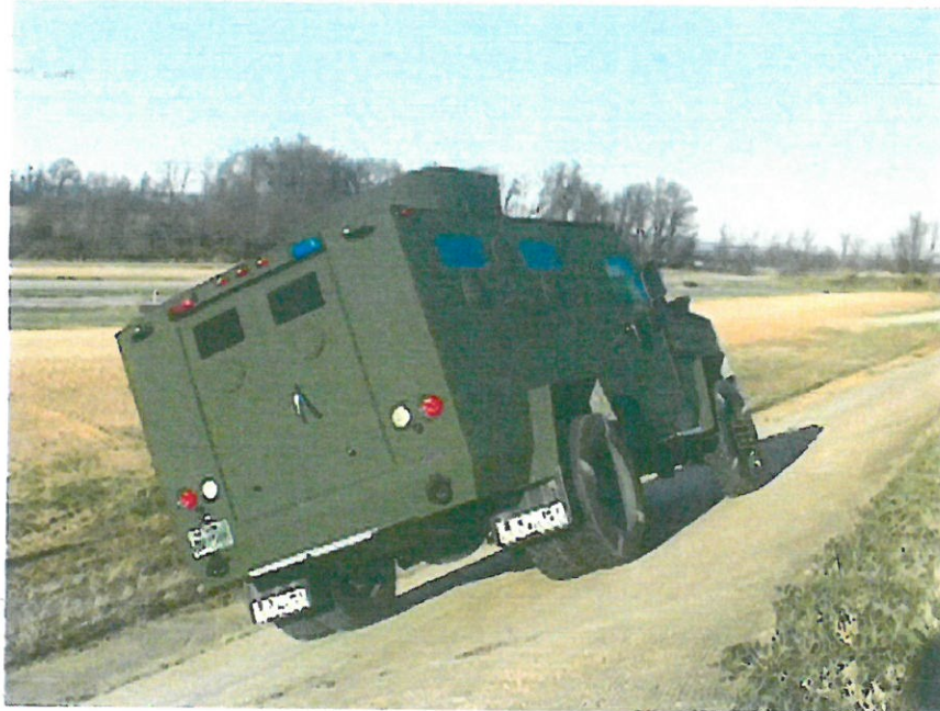
Figure 7. The BearCat negotiating the 40-percent side slope.
