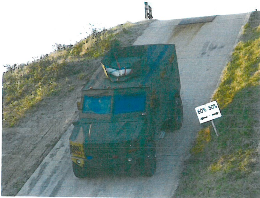
Figure 5. The BearCat descending the 60-percent longitudinal grade.
