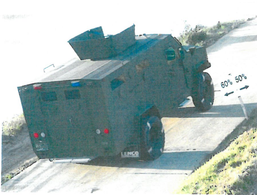
Figure 4. The BearCat ascending the 60-percent longitudinal grade.
