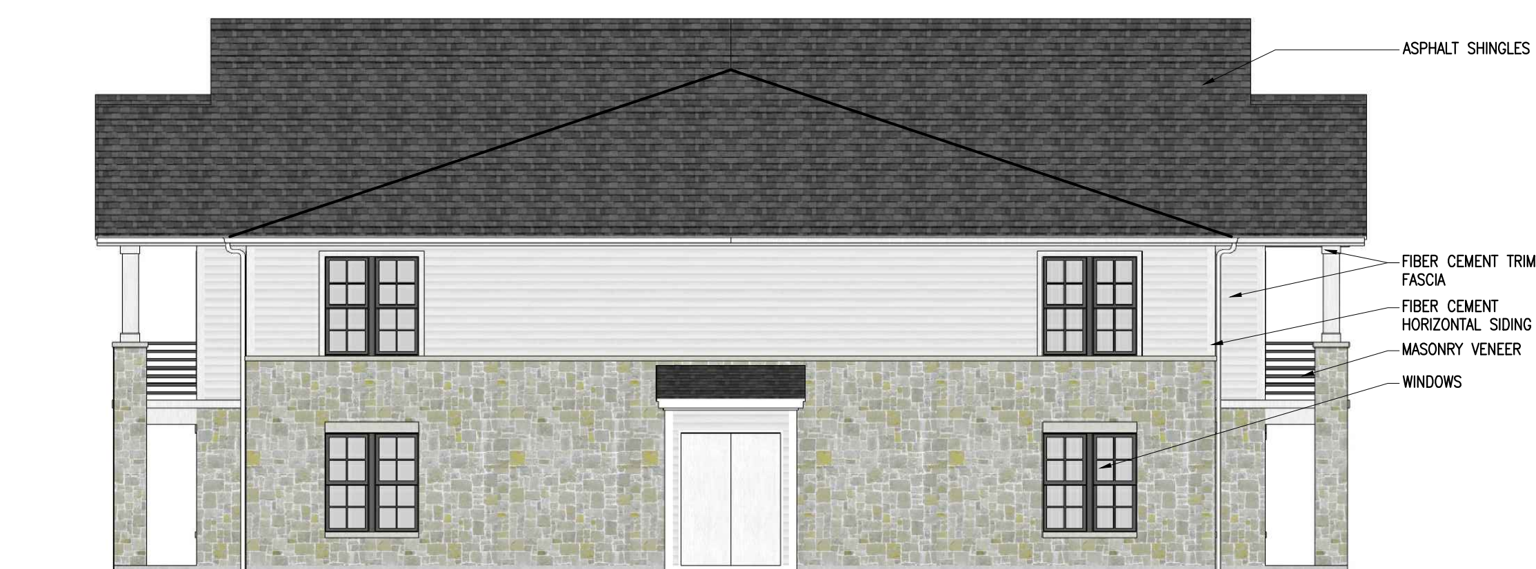
22 UNIT BUILDING - TYPE 'B' RIGHT ELEVATION 1/8" = 1'-0"
