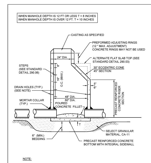
A MINIMUM OF 4 PRECAST OR DRILLED 1" DIAMETER HOLES SHALL BE PROVIDED WITHIN 1' OF THE LOWEST PIPE INVERT. THE HOLES SHALL BE DISTRIBUTED EQUIDISTANT AROUND THE PERIMETER OF THE STRUCTURE. A 1' BY 1' SQUARE OF UNDERDRAIN FILTER CLOTH MATERIAL SHALL BE FIXED OVER EACH DRAIN HOLE ON THE OUTSIDE OF THE STRUCTURE WITH MASTIC MATERIAL TO PREVENT SLIPPAGE DURING BACKFILLING.
