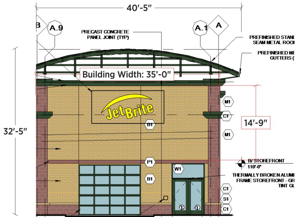
**SOUTH ELEVATION SCALE 3/32"=1'**
