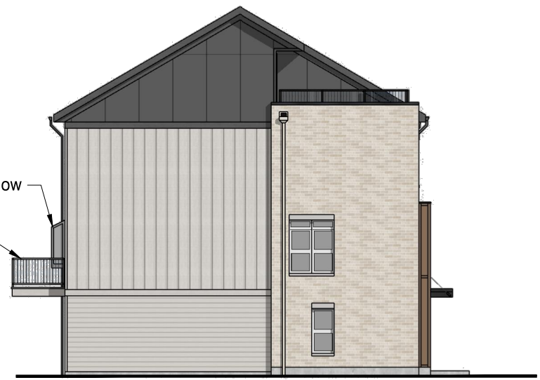
Left Elevation 1/16" = 1' Brick Coverage: 34%
