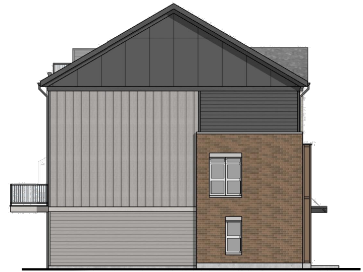
Left Elevation 1/16" = 1' Brick Coverage: 22%
