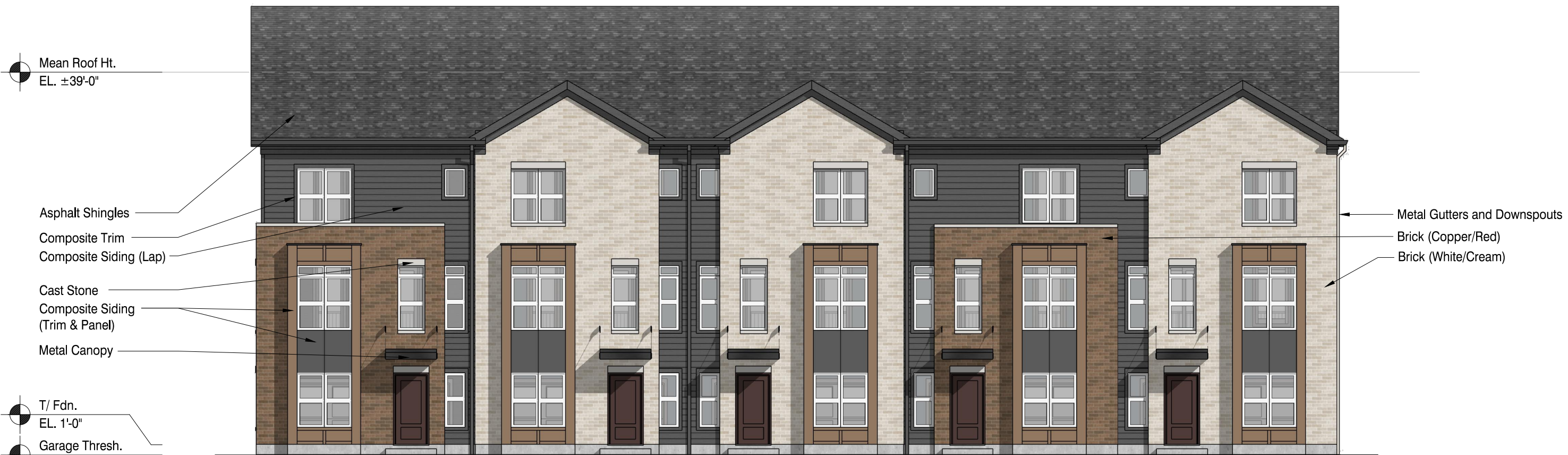
Front Elevation Color Scheme A 1" = 10' Brick Coverage: 62% Total Brick Coverage: 30%
