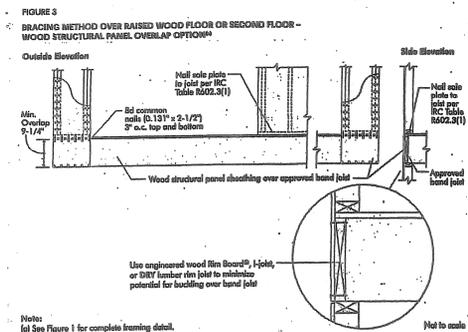
FIGURE 3 BRACING METHOD OVER RAISED WOOD FLOOR OR SECOND FLOOR WOOD STRUCTURAL PANEL OVERBAY CORNER
