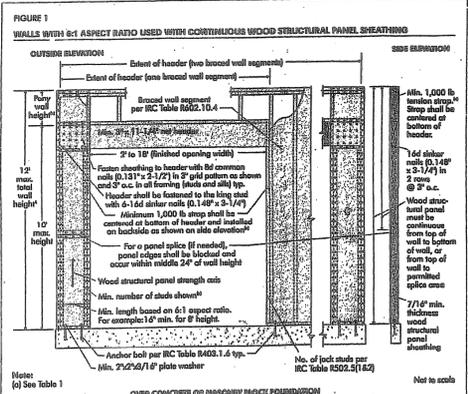
FIGURE 1 WALLS WITH 1:1 ASPECT RATIO USED WITH CONTINUOUS WOOD STRUCTURAL PANEL SHEATHING
