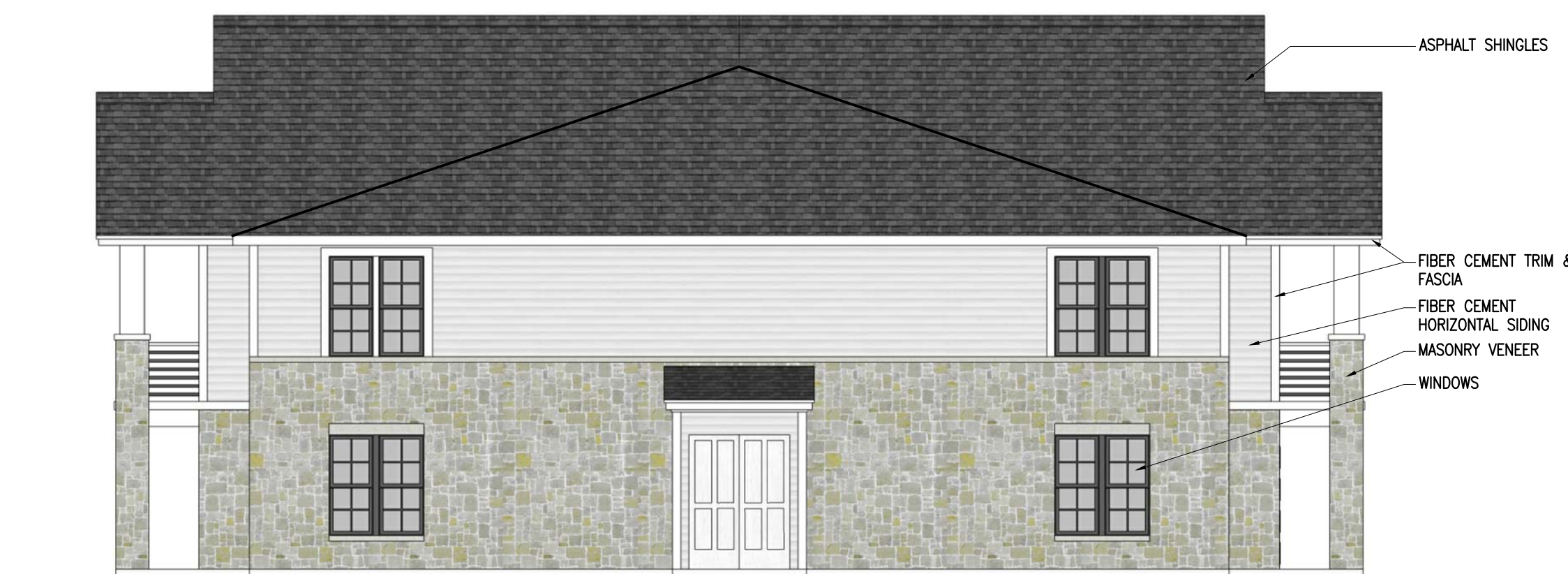
TYPICAL 18 UNIT BUILDING LEFT ELEVATION 1/8" = 1'-0"
