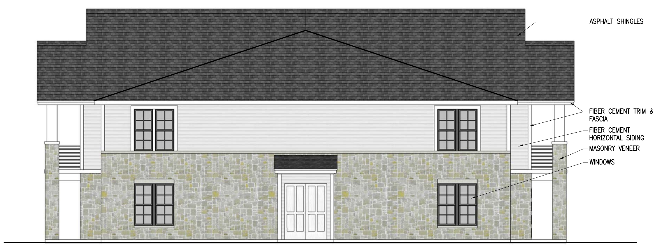
TYPICAL 22 UNIT BUILDING LEFT ELEVATION 1/8" = 1'-0"
