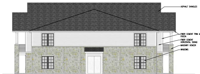
18 UNIT BUILDING - TYPE 'C' LEFT ELEVATION 1/8" = 1'-0"
