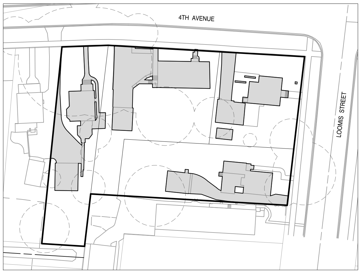
EXISTING PERVIOUS/IMPERVIOUS CONDITIONS 1"=50'
