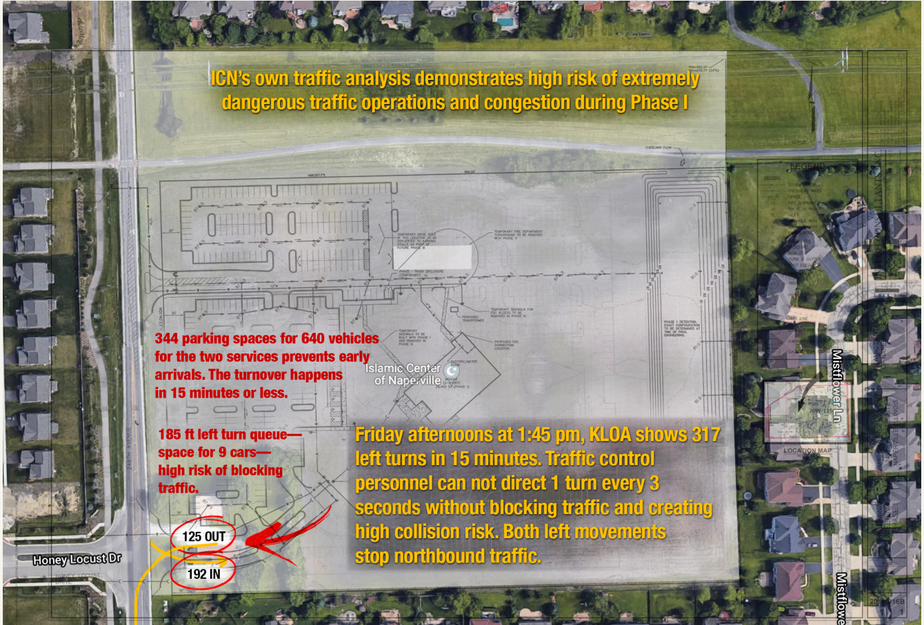
Figure 3: Graphic above illustrates left turns only and hazardous operational conditions.
