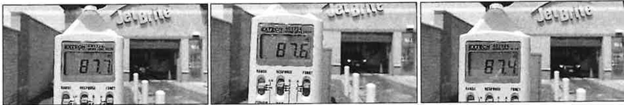
Photo 2: Noise readings – Car wash side of wall
