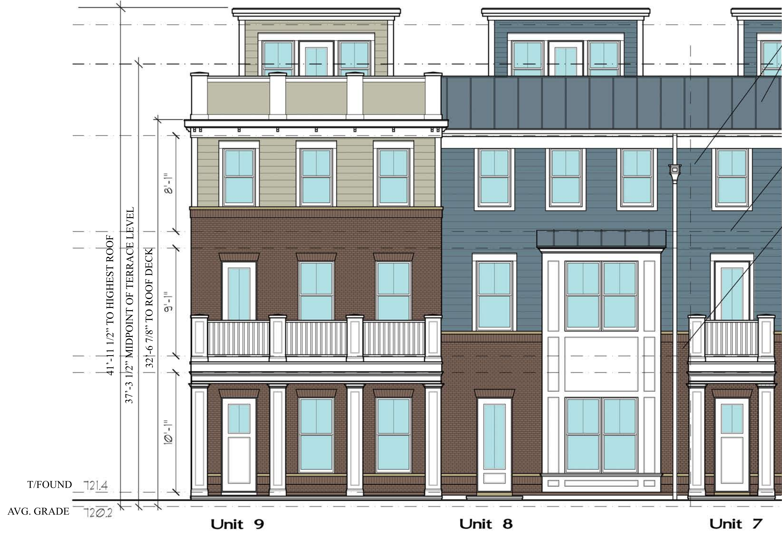
3 PI 4th Avenue Elevation Detail (North) SCALE: 1/4" = 1'-0"
