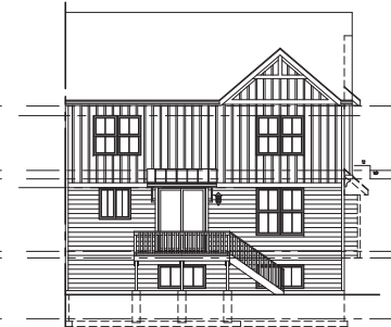
REAR ELEVATION - THE NAPER SCALE: 1/8" = 1'-0" LOOK-OUT BASEMENT
