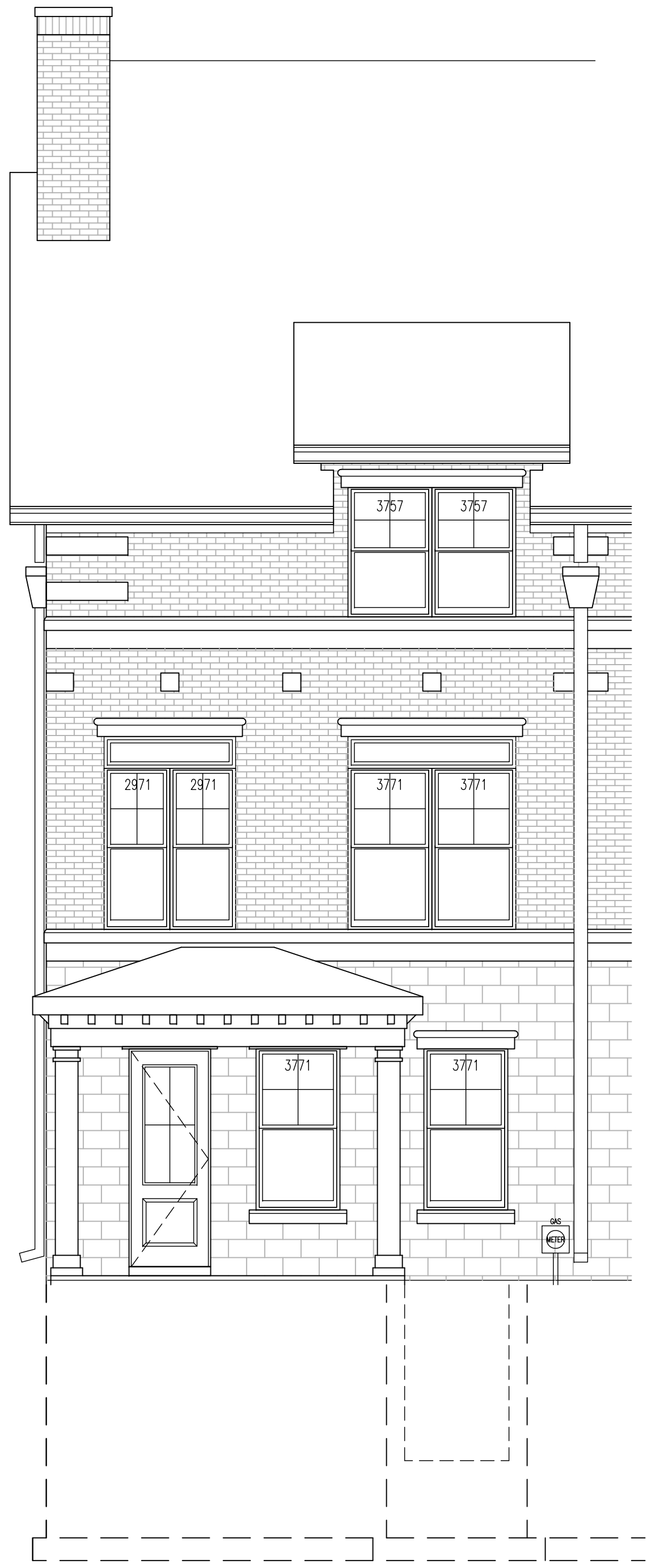
H FRONT ELEVATION - H 1/4" = 1'-0"
