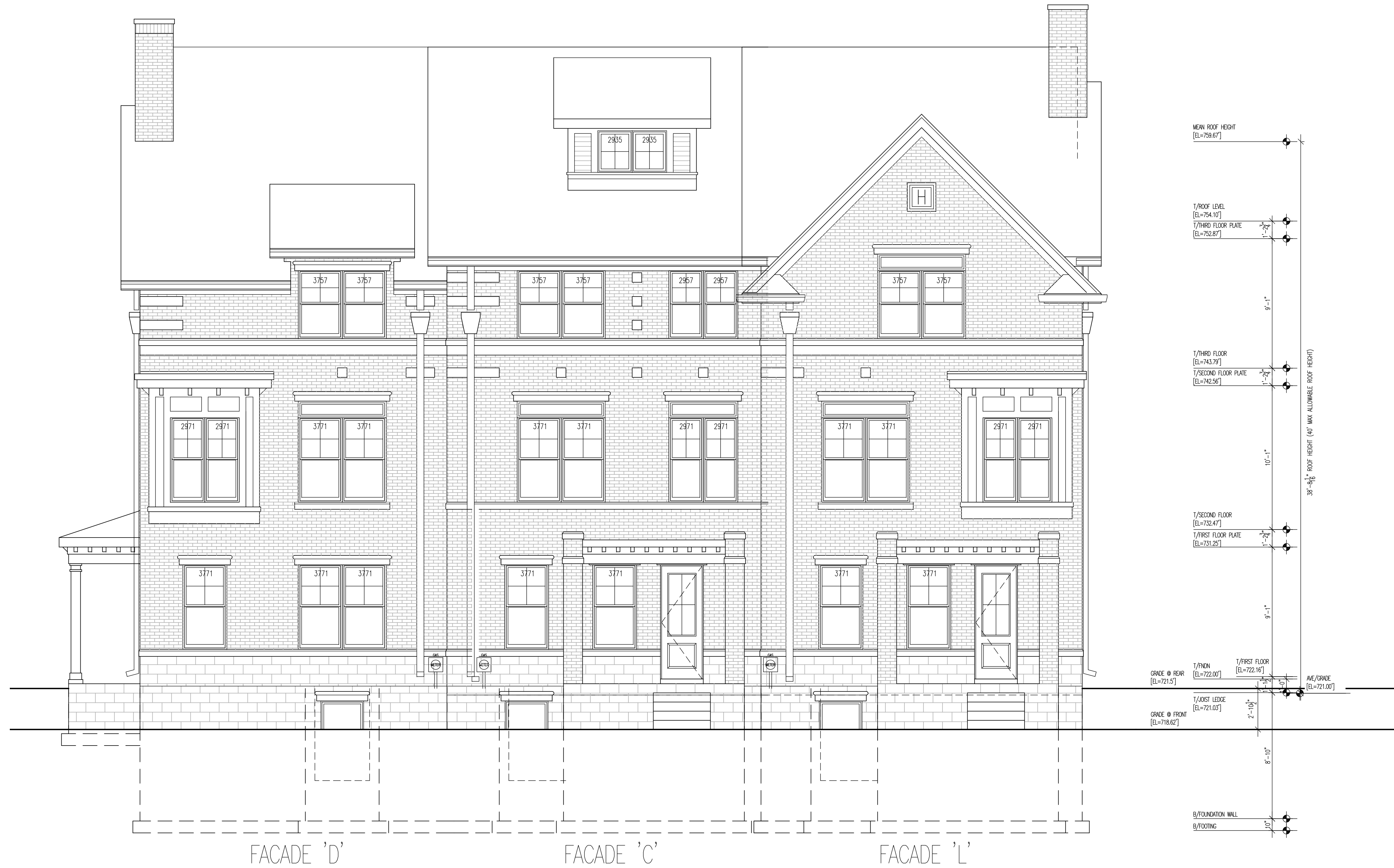
2 FRONT ELEVATION - BUILDING 2 1/4" = 1'-0"
