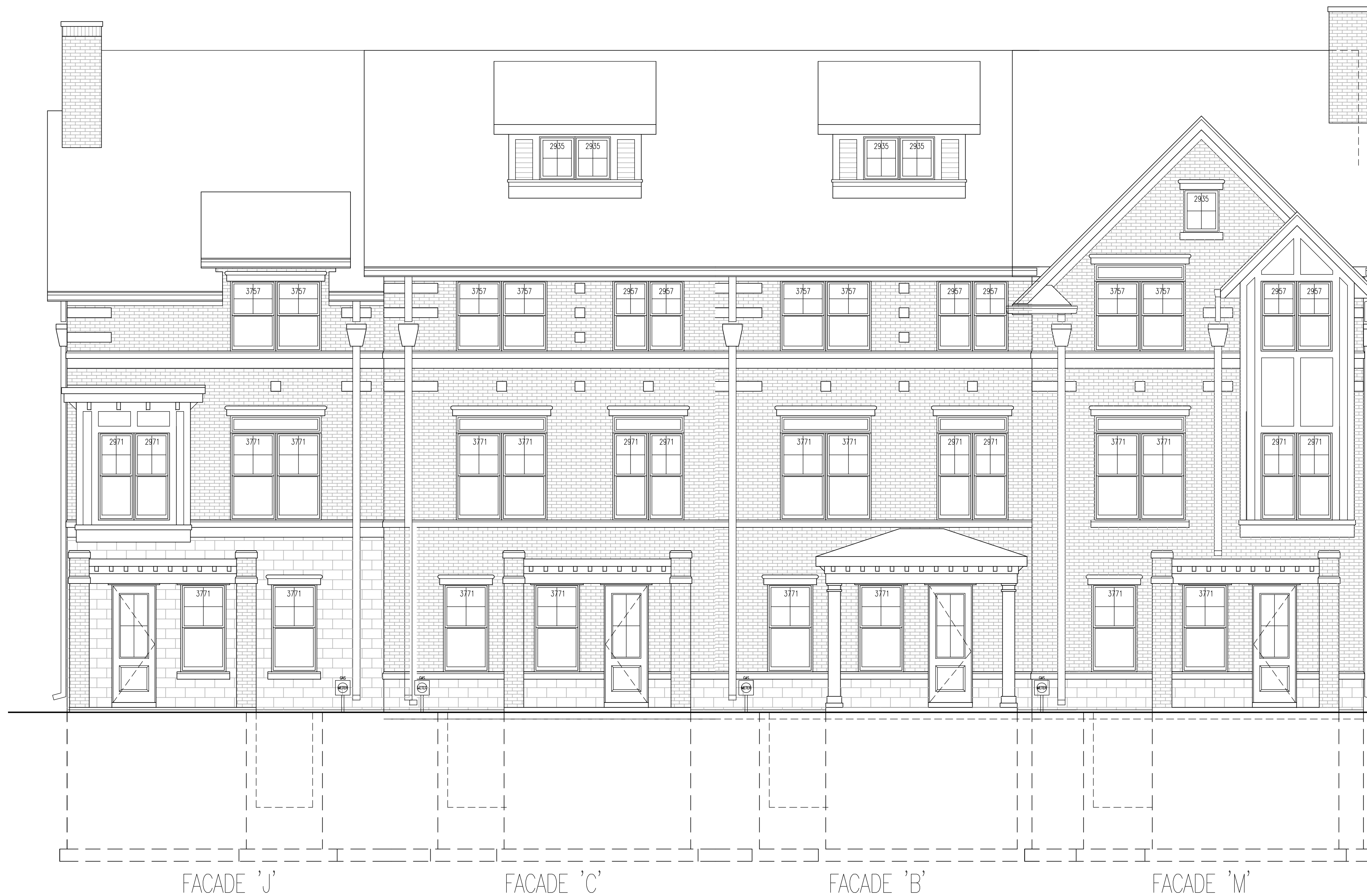
8 FRONT ELEVATION - BUILDING 8 1/4" = 1'-0"
