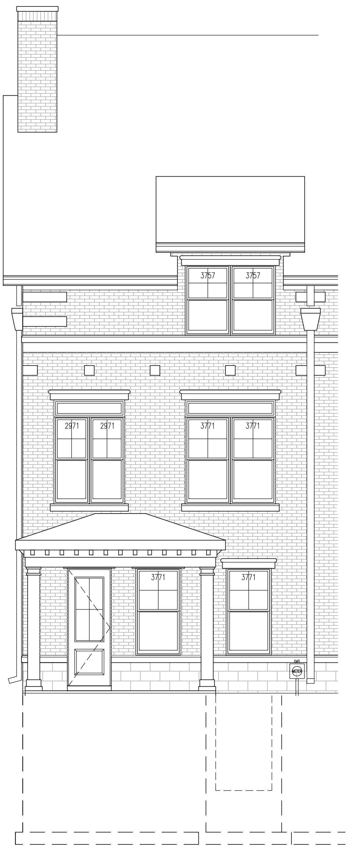
F FRONT ELEVATION - F 1/4" = 1'-0"
