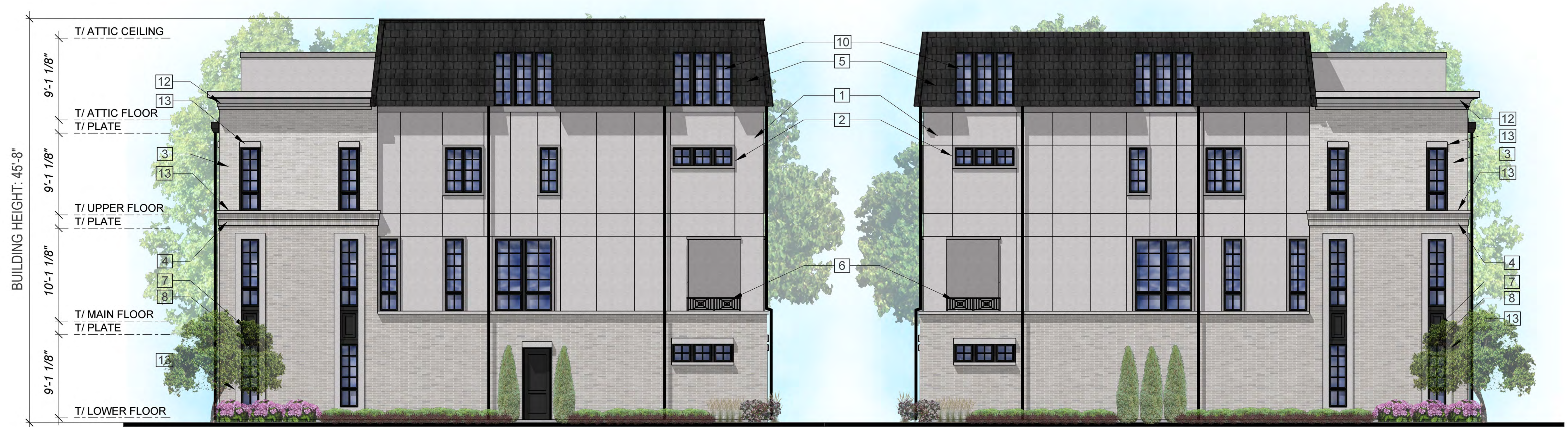
Masonry: 100% Right Elevation Scale: 3/16" = 1'-0"
