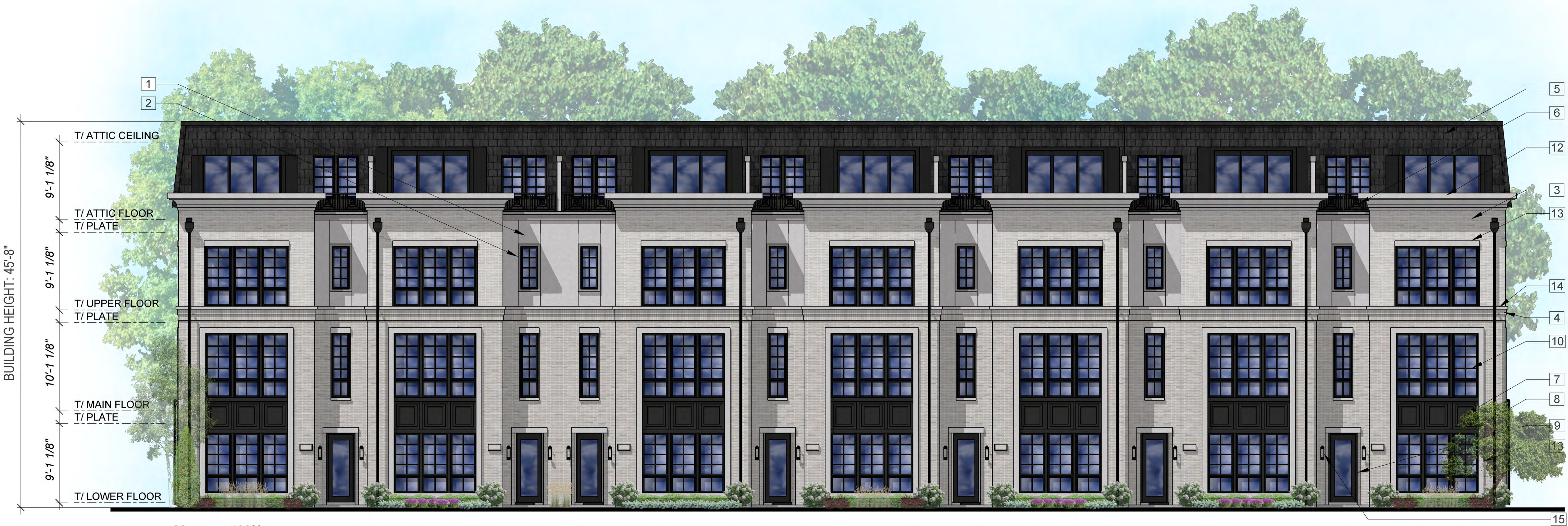
Masonry: 100% Front Elevation Scale: 3/16" = 1'-0"
