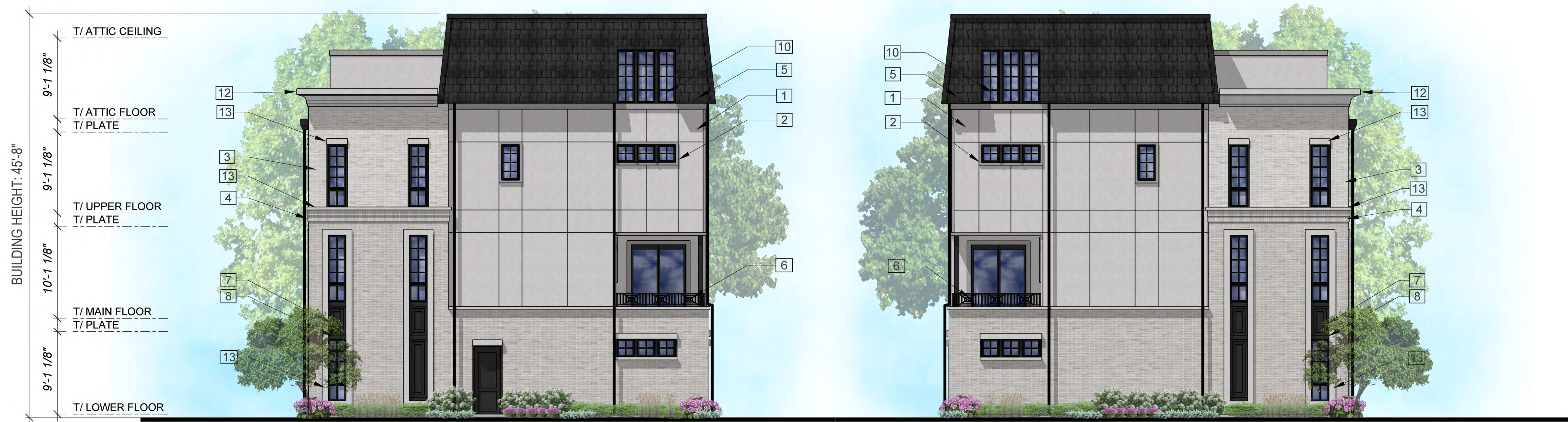
Masonry: 100% Right Elevation Scale: 3/16" = 1'-0"
