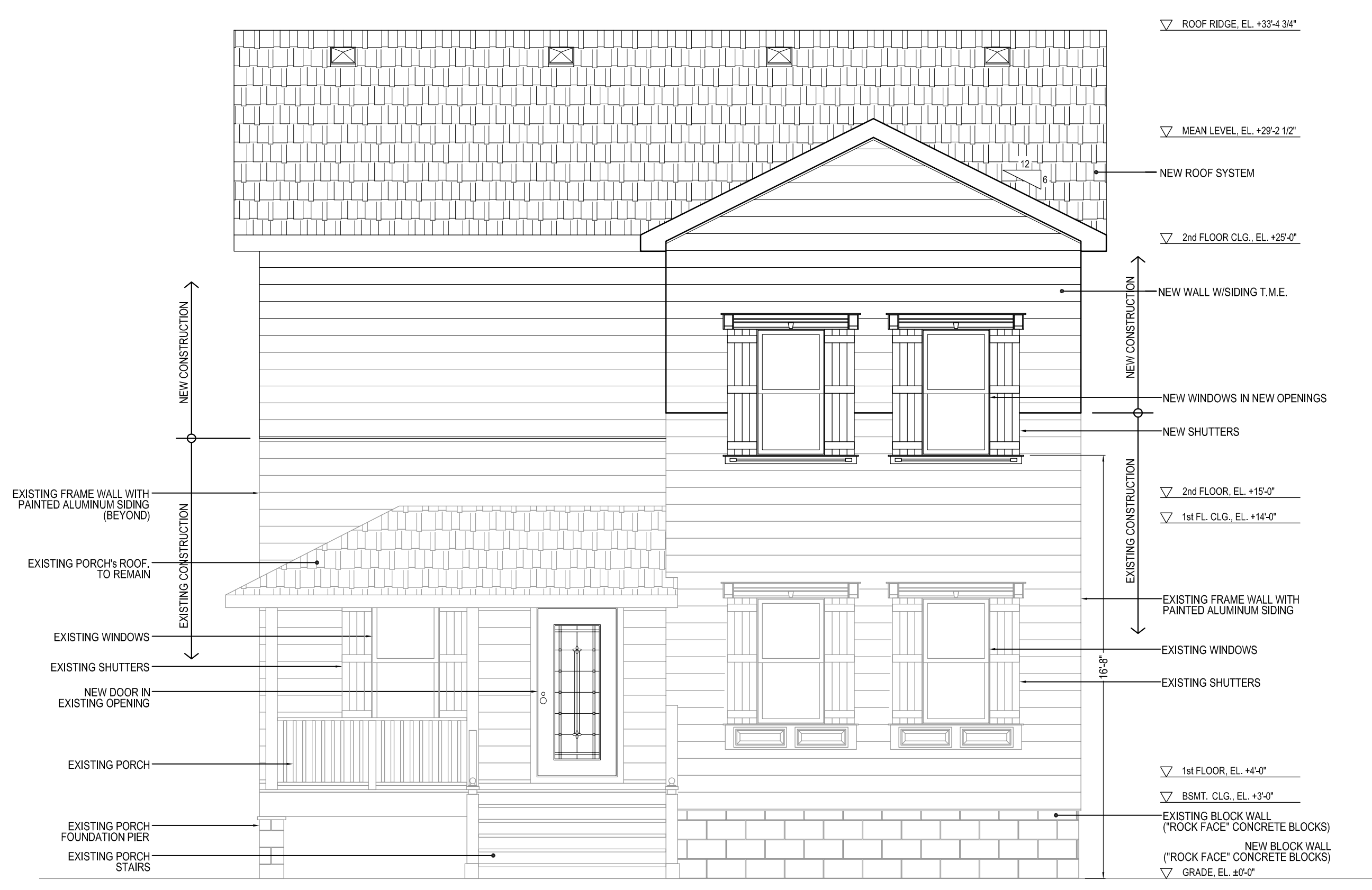
1 PROPOSED EAST ELEVATION (FRONT ELEVATION) SCALE 1/4"=1'-0"
