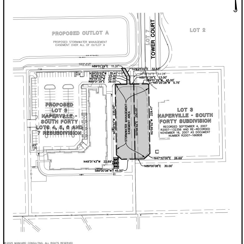
THE STORMWATER FACILITY AND EASEMENT
