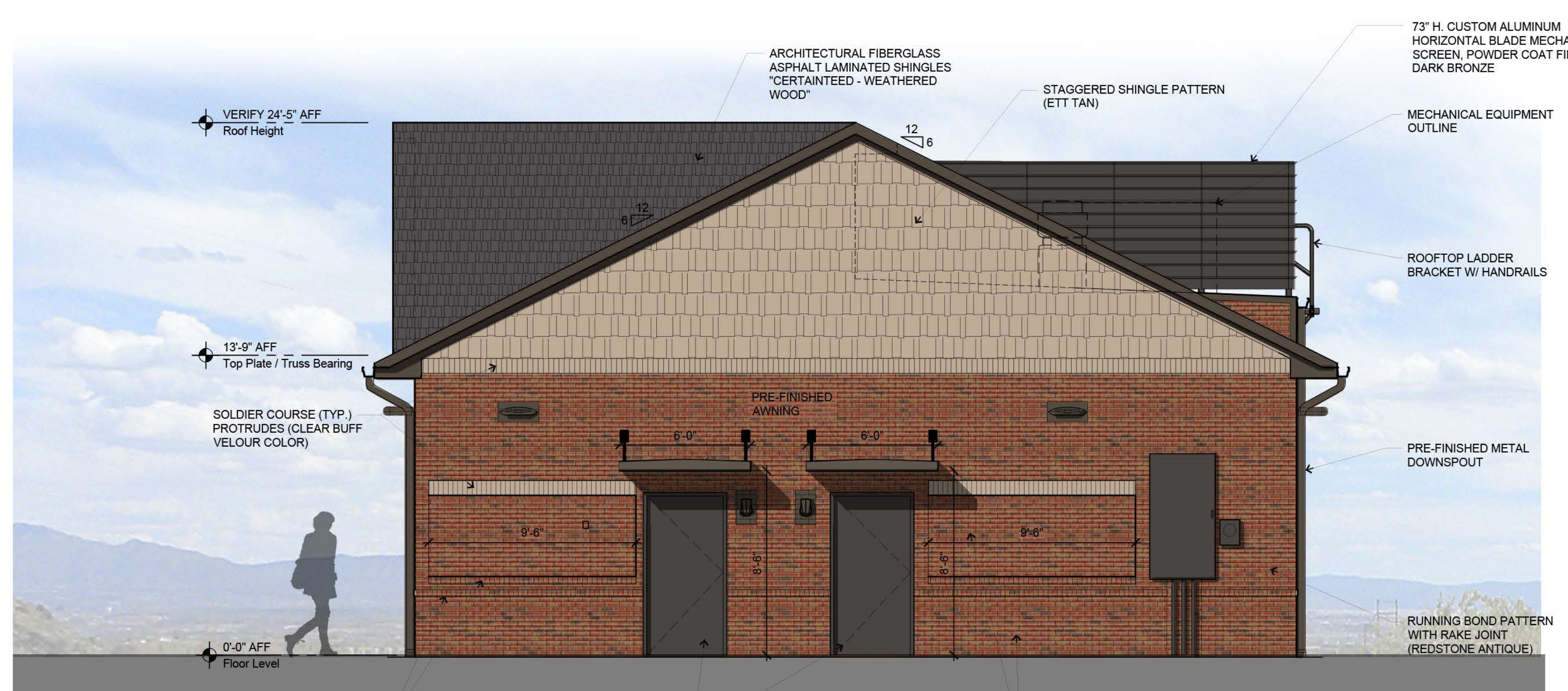
1 Exterior Elevation - Back of Building (Plan North) 1/4"=1'-0"
