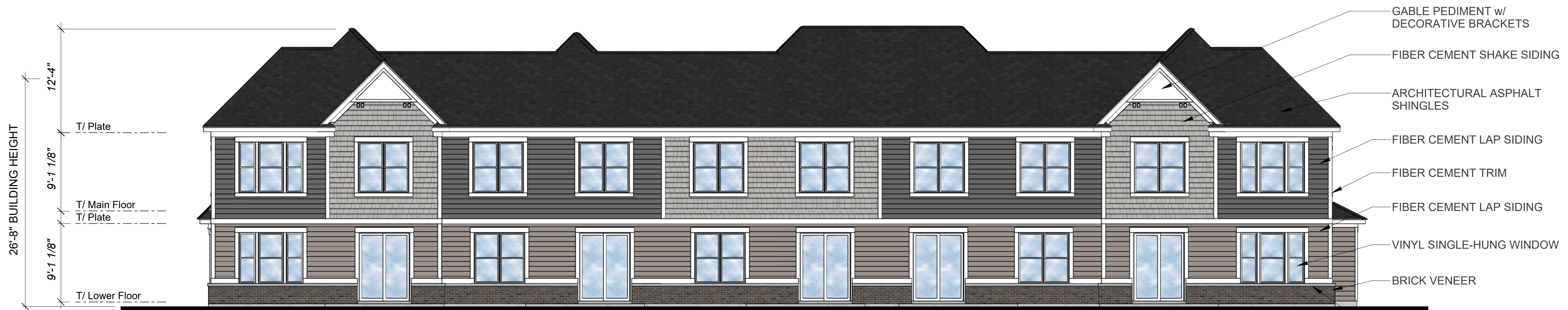
Masonry: 100% Rear Elevation Scale: 3/16" = 1'-0"
