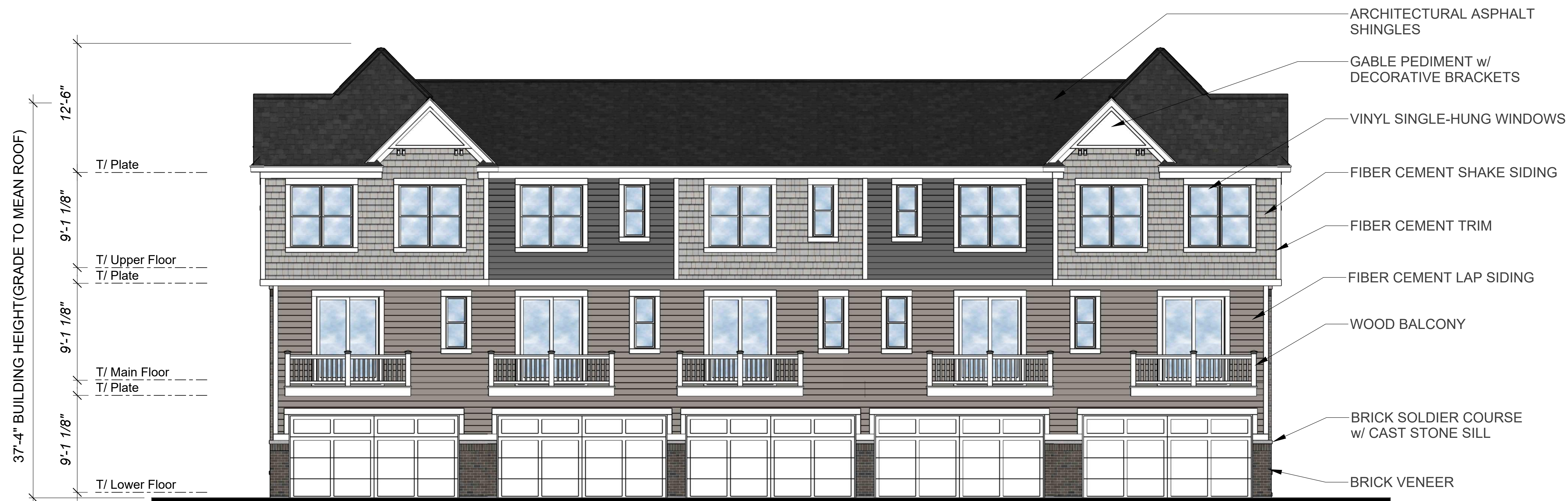
Masonry: 100% Rear Elevation Scale: 3/16" = 1'-0"
