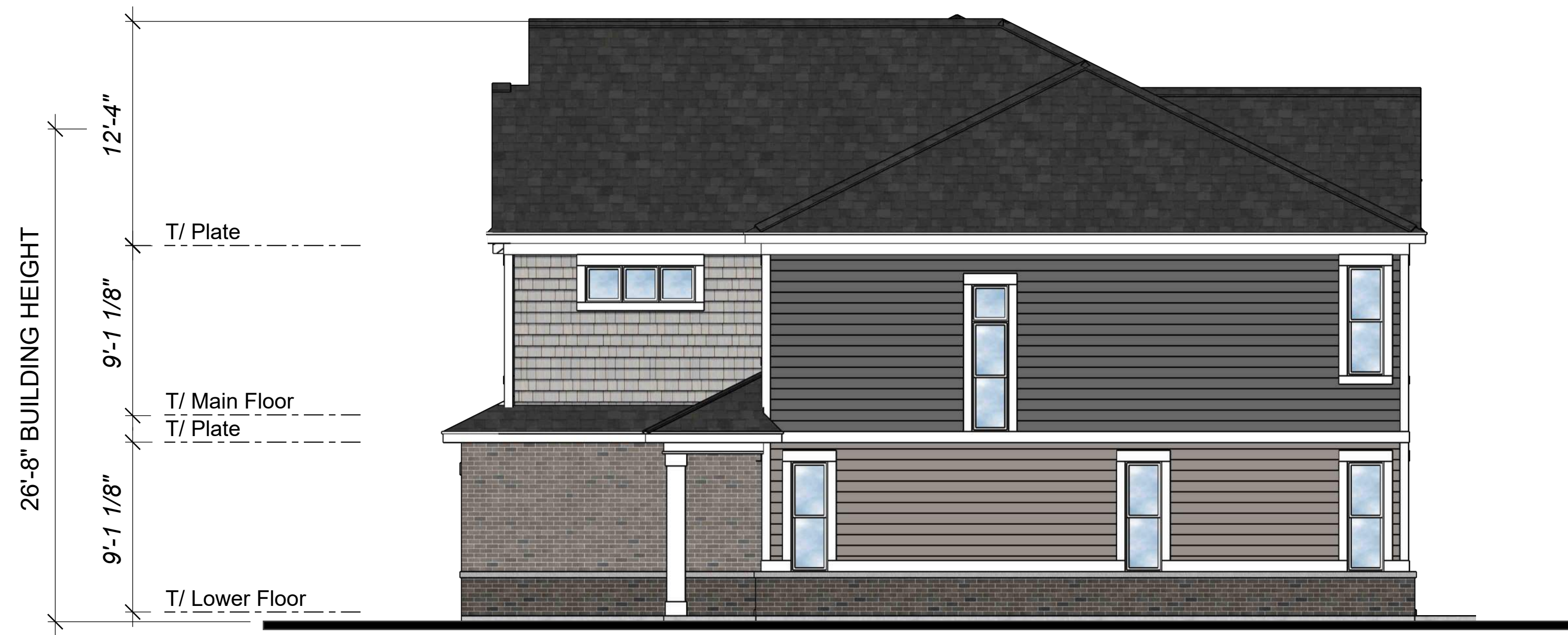
Masonry: 100% Typical Side Elevation Scale: 3/16" = 1'-0"
