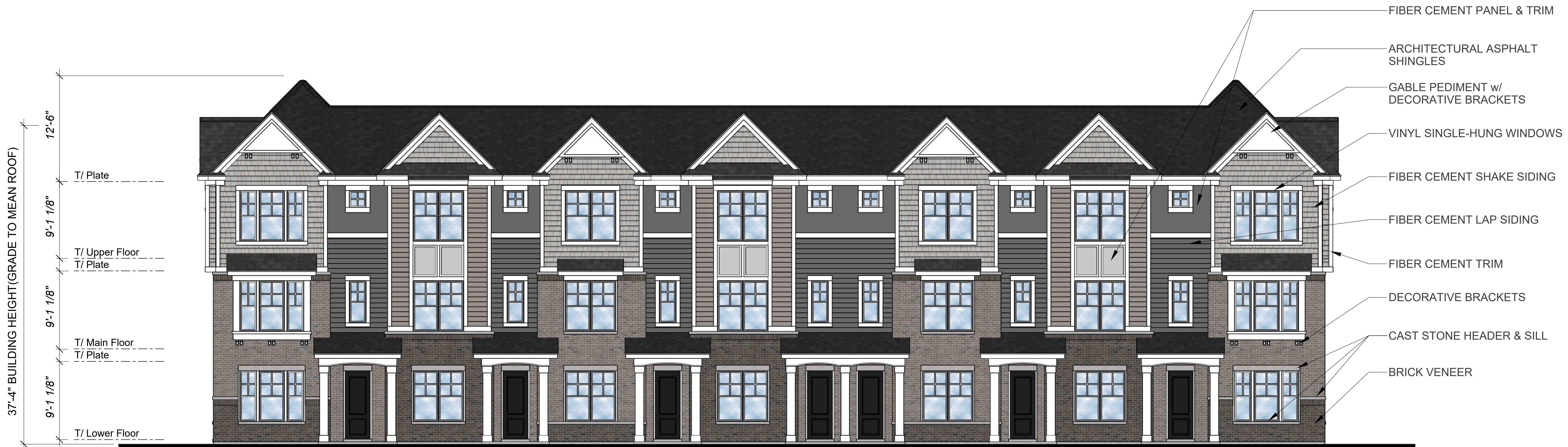
Masonry: 100% Front Elevation Scale: 3/16" = 1'-0"
