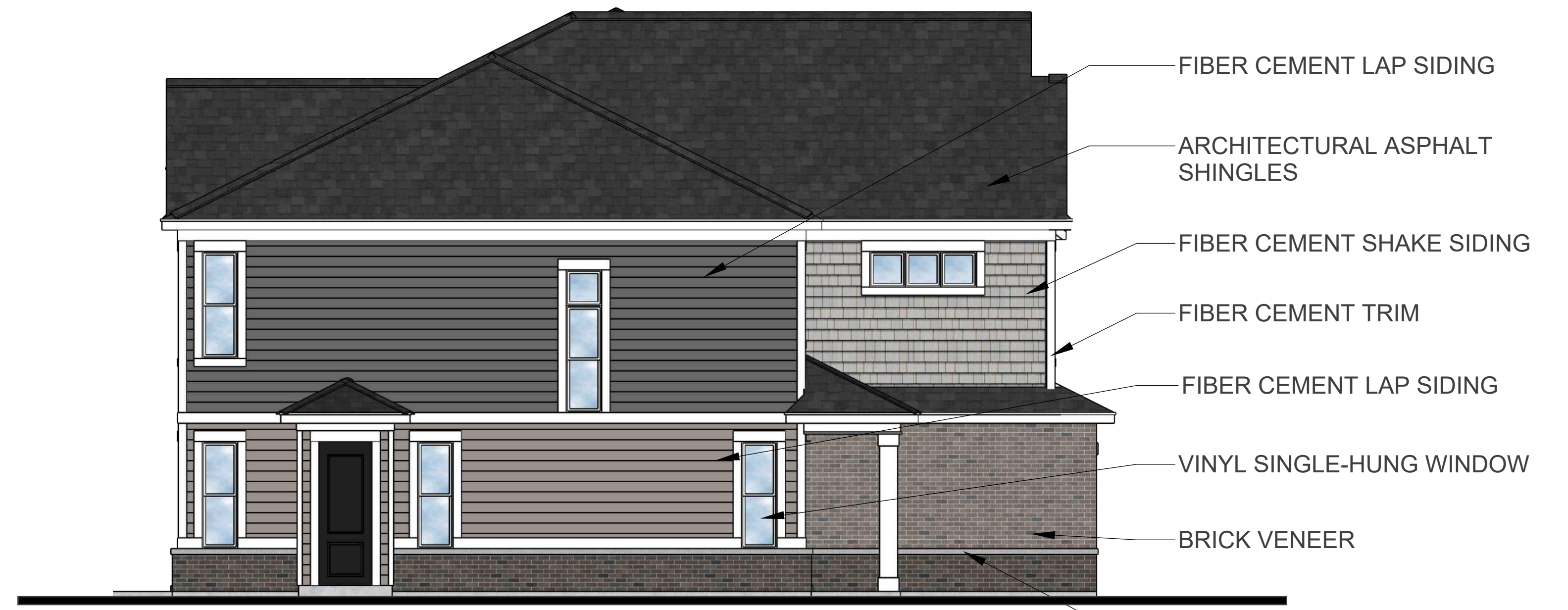
Masonry: 100% Side Elevation (FACP) Scale: 3/16" = 1'-0"
