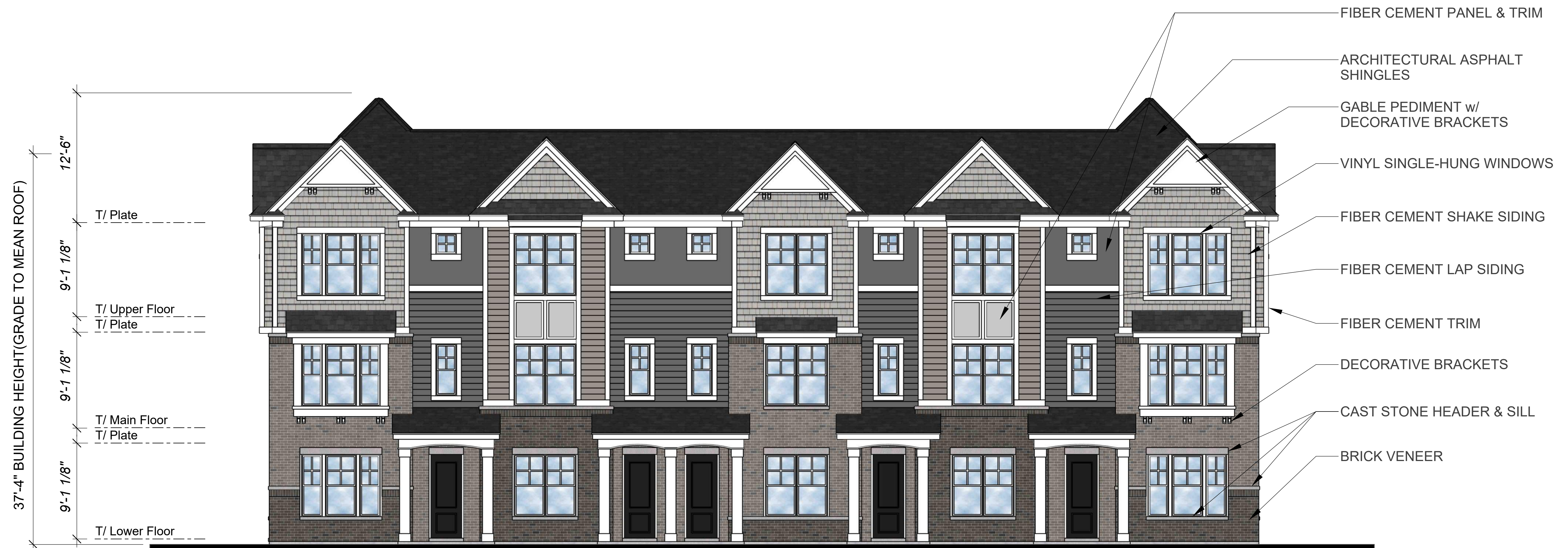
Masonry: 100% Front Elevation Scale: 3/16" = 1'-0"
