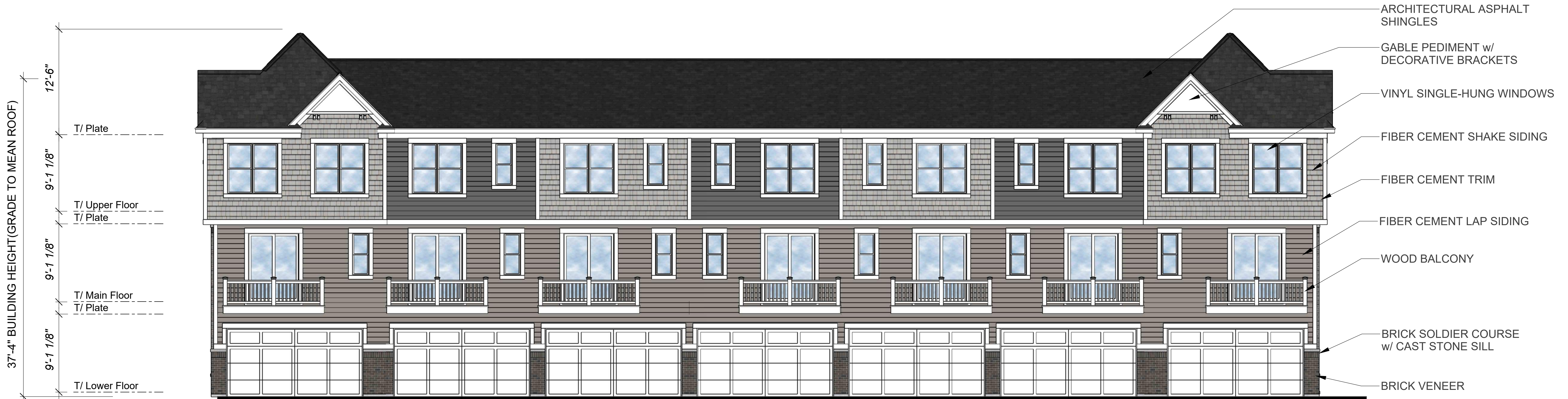
Masonry: 100% Rear Elevation Scale: 3/16" = 1'-0"
