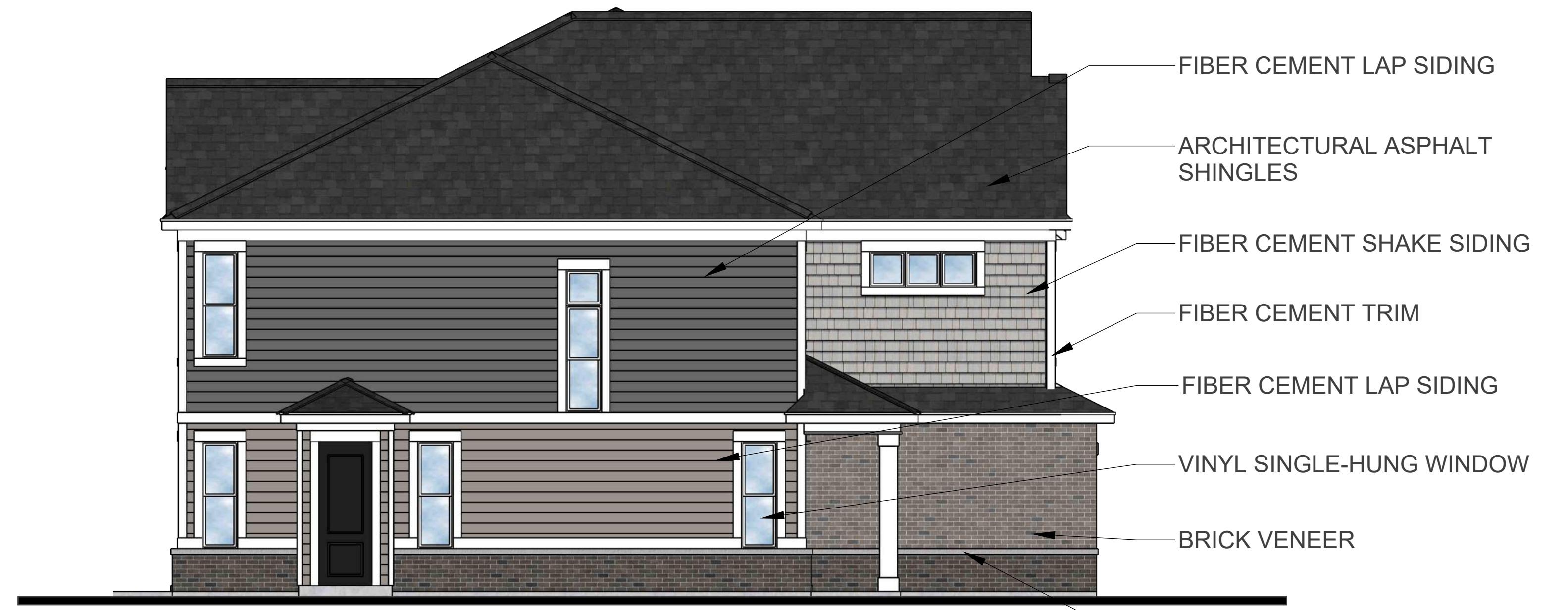
Masonry: 100% Side Elevation (FACP) Scale: 3/16" = 1'-0"
