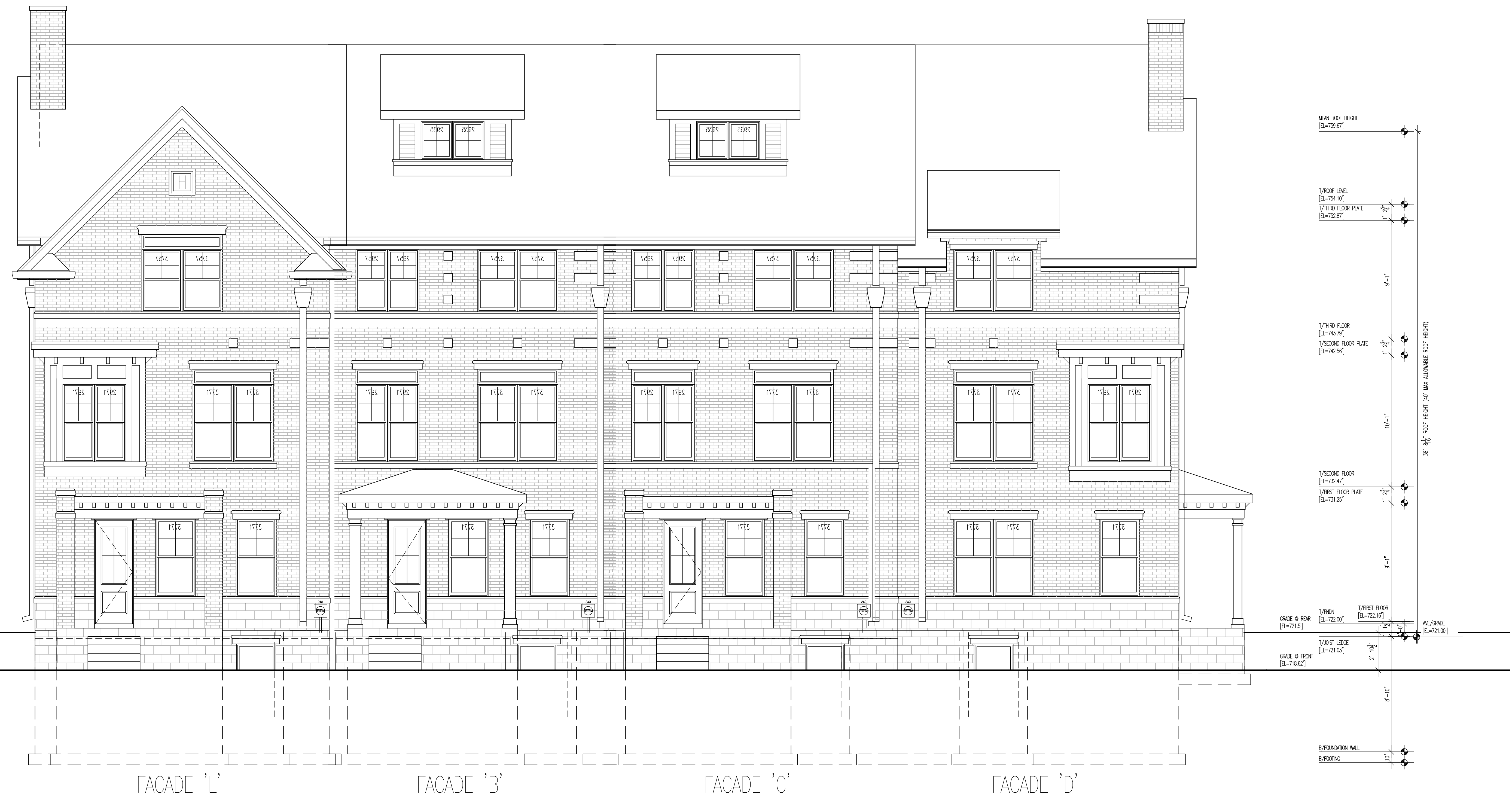
4 FRONT ELEVATION - BUILDING 4 1/4" = 1'-0"
