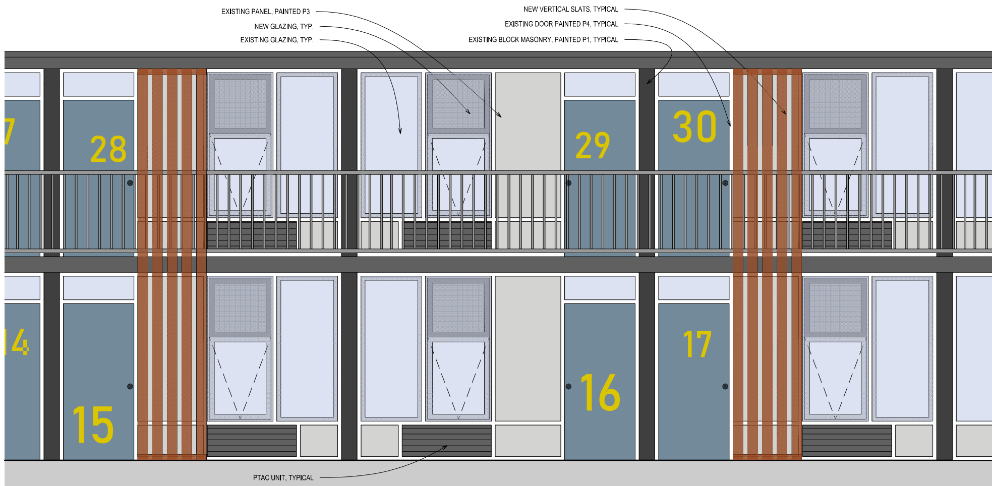
1 WEST ELEVATION DETAIL SCALE: 3/8" = 1'-0"
