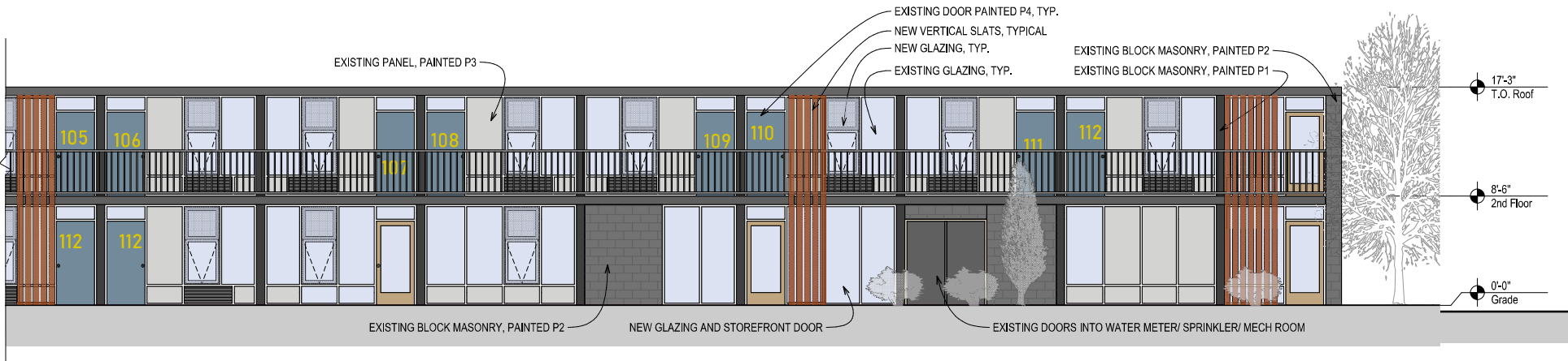
2 Proposed East Elevation SCALE: 1/8" = 1'-0"
