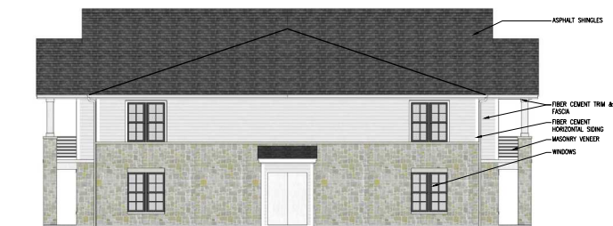
22 UNIT BUILDING - TYPE 'A' RIGHT ELEVATION 1/8" = 1'-0"
