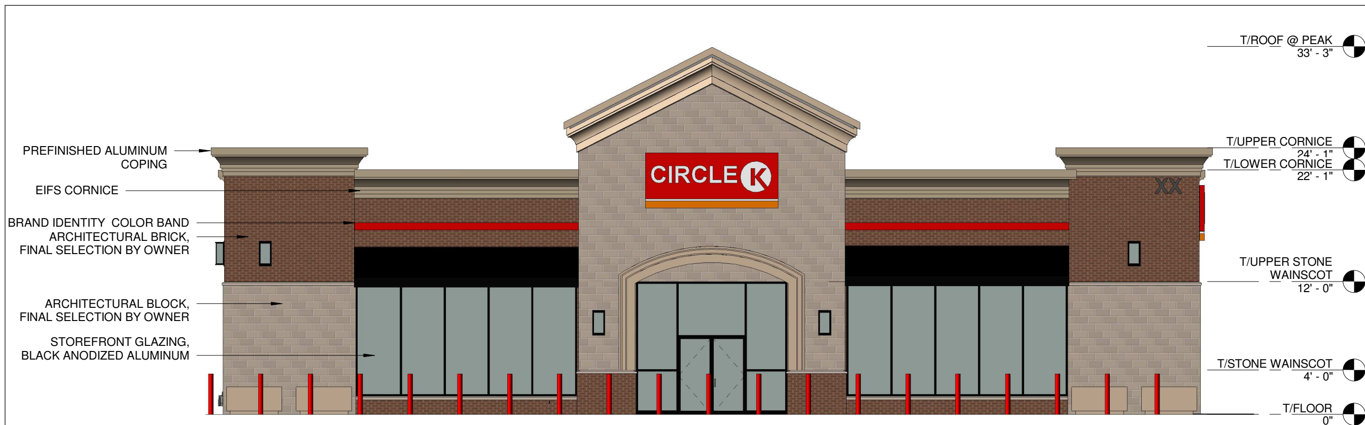
① FRONT ELEVATION 1/8" = 1'-0"
