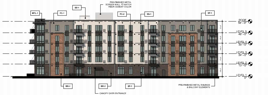
2 BUILDING ELEVATION - WEST 1/16" = 1'-0"
