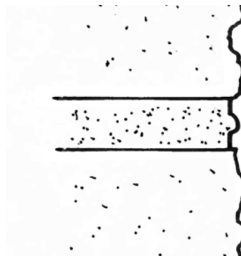
Illustration D.5 - Beaded mortar joint profile, typical of stone masonry in the Historic District
