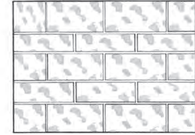
Illustration D.4 - Stamped concrete - rock face finish
